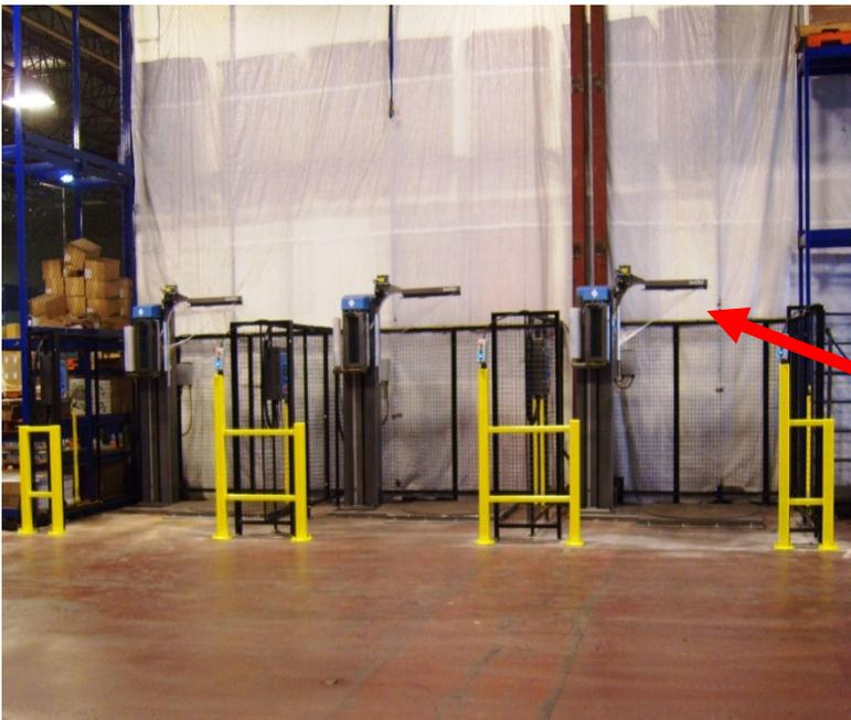
This photo shows three (3) Cousins A-Arm platform automatics installed in a strategic location. The layout allows the operator to place a pallet on a machine that is empty and be able to pick a pallet from a machine that has completed wrapping a pallet.
