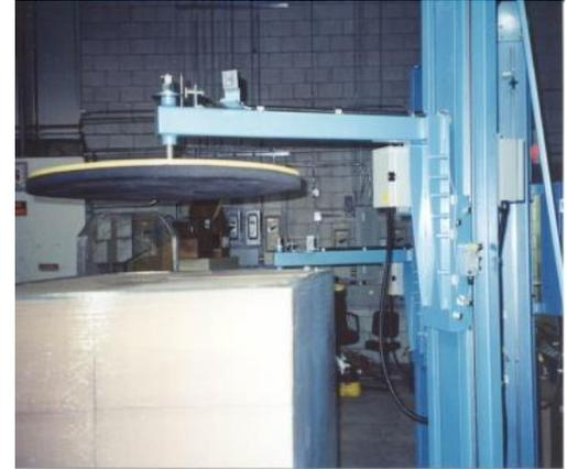
Top platens help stabilize the load during the wrap cycle
