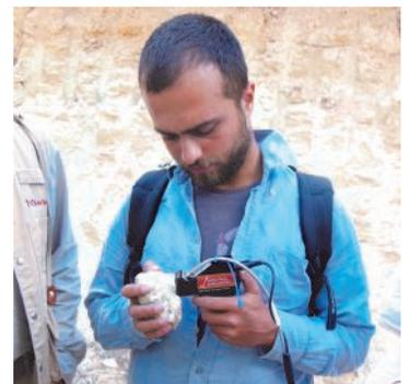
*The oreXpress is lightweight and easy-to-use, purpose-built for mining field work.*
