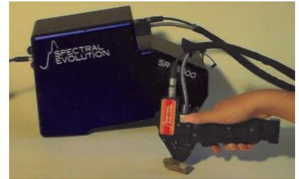
*SR-6500 ultra high resolution spectroradiometer with a MiniProbe for scanning small sample features.*
