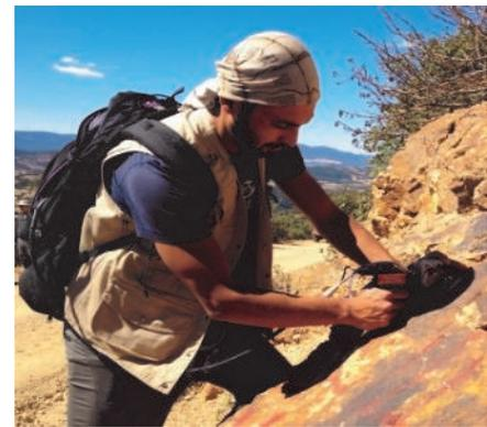
*SPECTRAL EVOLUTION's DAR-Win SP Data Acquisition software with EZ-ID and the Custom Library Builder module provides for mineral identification in the field to help in oil and gas exploration.*
