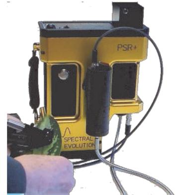
*The PSR+ is lightweight and portable for in situ measurements and plant identification.*
