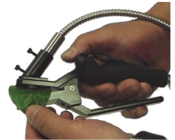
*Unique leaf clip protects your sample from heat and damage during scanning.*
