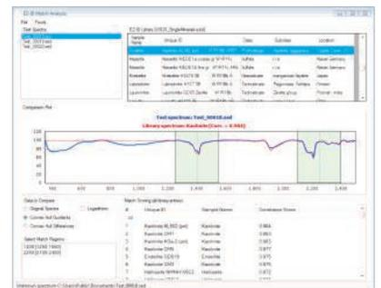
*EZ-ID screen with a scan of kaolinite. Kaolinite is a soft mineral that affects ore processing. It has been identified here using the USGS library.*
