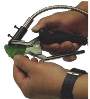
*An optional leaf clip includes an internal reference standard and an external trigger*
