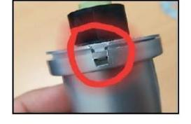
**STEP 3:** Now connect the upper part of the dongle back to the inverter as shown. (Important Step)
