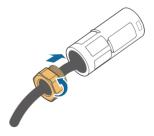
2. Put the locking ring into the housing.
