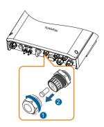
2. Lead the cable through the cable gland.
