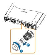
2. Lead the cable through the cable gland.
