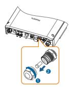
Lead the cable through the cable gland.
