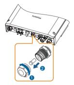
3. Lead the cable through the cable gland.
