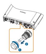
Lead the cable through the cable gland and remove the cable jacket by 8 mm-15 mm.
