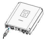
6. Connect the other ends to the emergency loads. Pull all the lines outward to check whether they are firmly installed.
