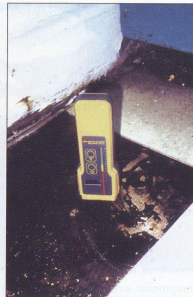
A portable moisture meter can help accurately identify moisture levels and uncover potential for mold growth.
