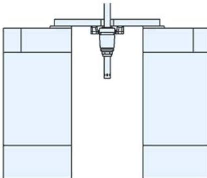
When installing a new blow pin assembly, and with the mold clamp in the open position, place the tool across the top of both mold halves. Be sure that the tool is resting on the top of the shear steels and not on the top blocks. The ends of the tool have a radius that matches the pocket in the top of the top blocks in case your shear steels sit below the top of the top block.
