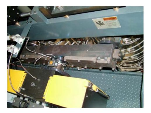
**New Divider Manifold with Plate Heaters and Shutoff Valve**
