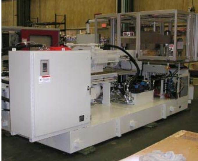
AC Variable Frequency Drive Package Installed on an IBS-122 Machine
