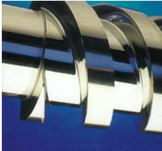
One of the most common causes of poor extruder function is excessive barrel and screw wear which leads to:
