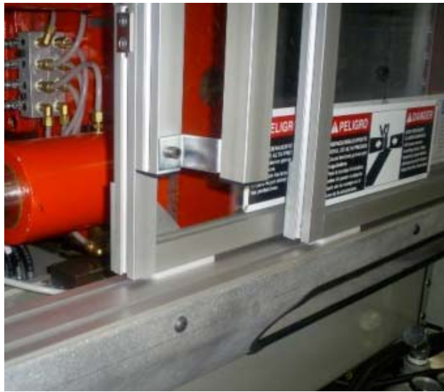
The Delrin slide pads can be seen between the bottom of the doors and the door frame.
