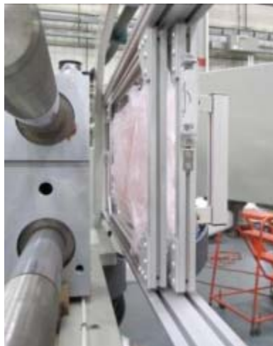
Transmitter mounting on the door and closure magnet plate.
