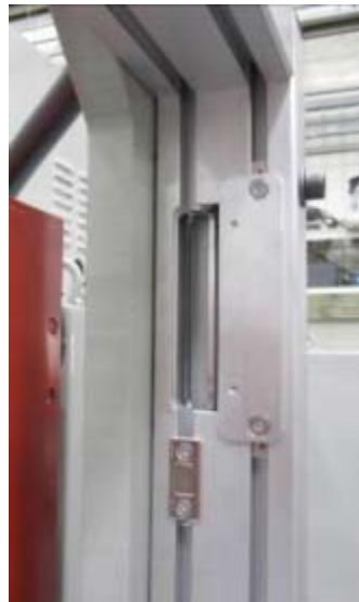
Switch mounting is recessed into door frame. Closure magnet is located just below the switch.
