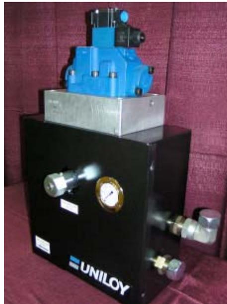
Uniloy is pleased to present this month's product offering; a high flow hydraulic valve assembly designed to take the place of the obsolete shot valve assemblies on your 350R4 and 400R machines.
