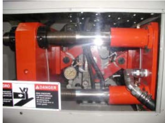
This package includes all of package A plus tie bar bushing retainers and platen shoes. The tie bar bushing retainers and shoes provide support and guidance for the linear motion of the platens. Worn tie bar bushings and shoes allow clamp misalignment which leads to increased mold wear and decreased blow molded product quality.
