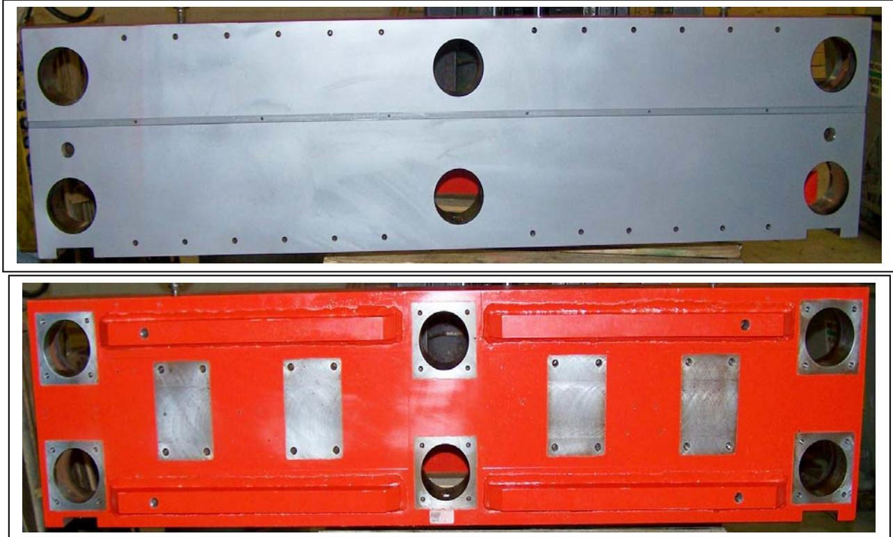
Uniloy is offering a platen exchange program for Reciprocating Screw machines. The key to this exchange program is that Uniloy has refurbished platens for most clamp sizes in stock and ready for shipment. Refurbished platens can be sent to you ready for install, minimizing machine down time.
