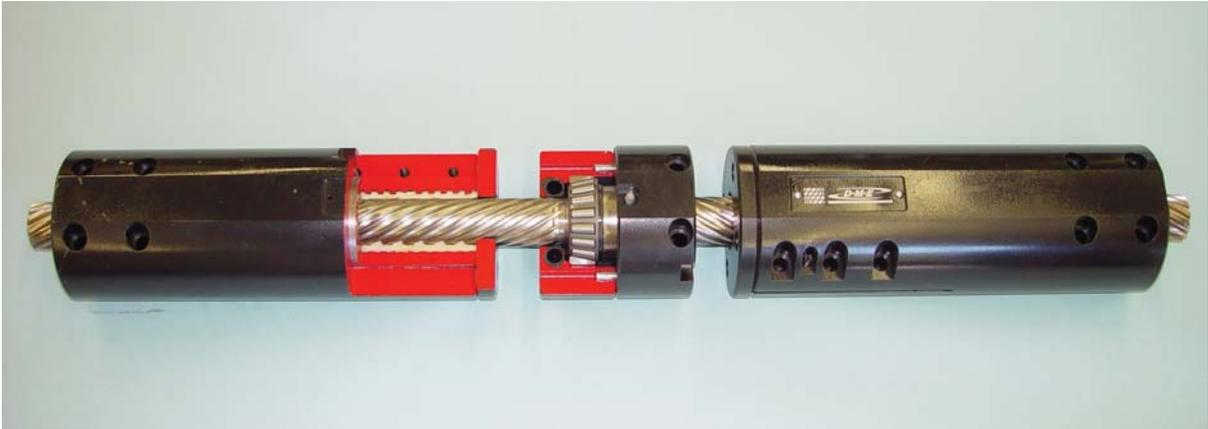
The function of the DME Helical Gear Stack Mold Centering Device is to provide equal and synchronized parting line openings for stack molds. The stack mold can be a standard, spin-stack or other type where centering of the center portion of the stack mold or center platen of a Dual Mold Carrier between the stationary and moving platen is required.
