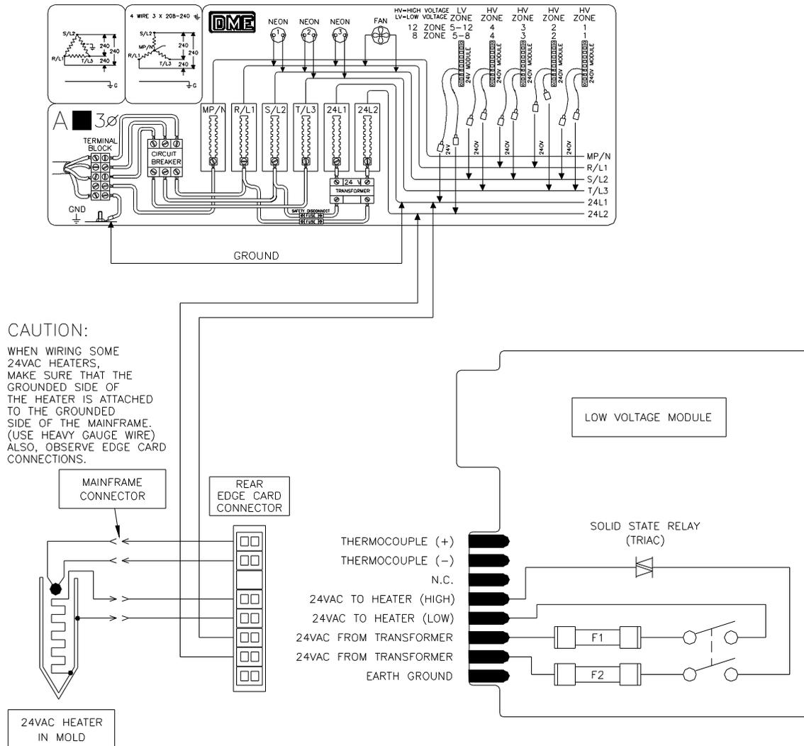
Figure 11 - Mold Wiring / Grounding
