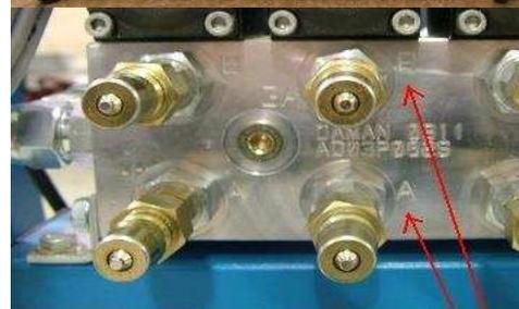
PORT "A" = PRESSURIZED WHEN TIMER ZONE IS "INACTIVE"
