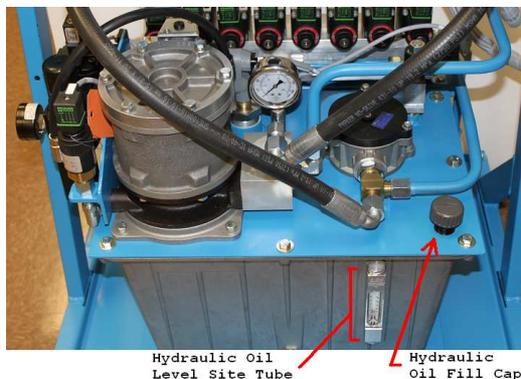
After making sure that the drain port on the front of the tank is tight, fill the reservoir to the top of the sight glass. Once the hydraulic connection lines are charged the first time, it may be necessary to add more hydraulic fluid.
