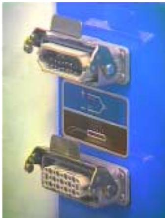
**Figure 1 - Power Connector (Bottom) & Thermocouple Connector (Top)**
