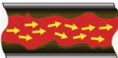
Partially Restricted flow of coolant
