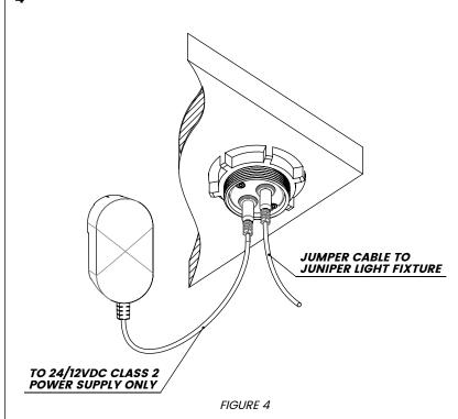
Connect the power supply as shown above. Connect the jumper cable to juniper lighting fixture.
