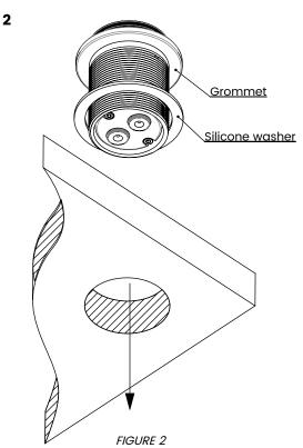
Slide the provided silicone washer on the grommet. Place the grommet in the hole.
