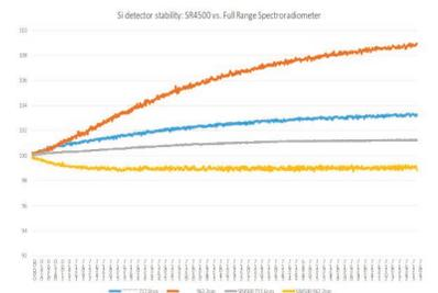
*Comparison of detector stability for an SR-4500 versus a typical full range spectroradiometer. Blue and orange lines represent the spectroradiometer; the gray and yellow the SR-4500.*
