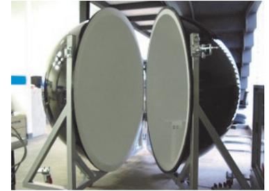
*Detailed calibrations using integrated spheres are used to fully characterize satellite instruments.*
