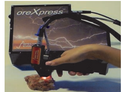
The oreXpress with the Miniprobe's 3mm spot size for field or core shack use.
