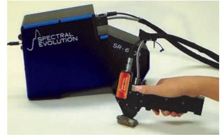
*SR-6500 delivers the highest available resolution for a portable spectrometer with a three TE-cooled photodiode array design.*
