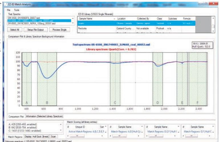
*The SR-6500 allows you to focus on absorption features that are just not apparent to a lower resolution instrument. With EZ-ID you can build your own library from known coal samples to match to target samples for fast identification.*
