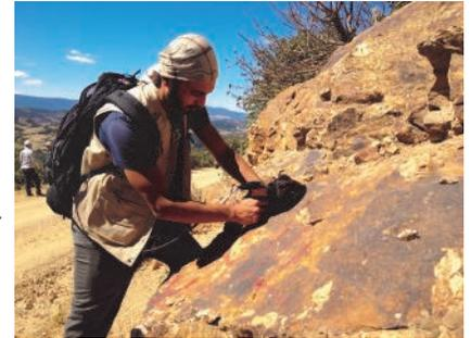
*oreXpress spectrometers are used to better understand and map mineral alteration zones in the field during exploration.*
