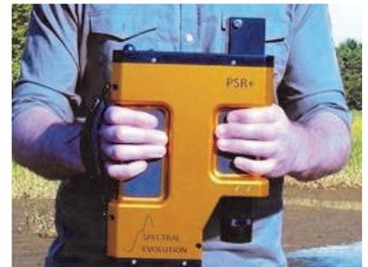
*The PSR + is a full range UV/VIS/ NIR, high resolution, field spectroradiometer for remote sensing applications including soil studies, water body research, climate studies, and vegetation research.*
