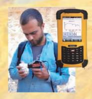
With the GETAC PS336 microcomputer and backpack, an oreXpress spectrometer is easy for one person to carry and operate in the field for rapidly collecting spectra on outcrops, blast hole chips, and hand samples.
