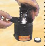
Many accessories are available including the benchtop lab reflectance probe with a scratchresistant sapphire window and a sample compactor for working with chips and powders.
