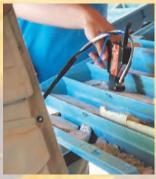
The oreXpress is also the instrument of choice for fast and accurate core logging. Spectra can be collected and minerals identified in real-time with EZ-ID or stored for later chemometric analysis using 3rd party software.
