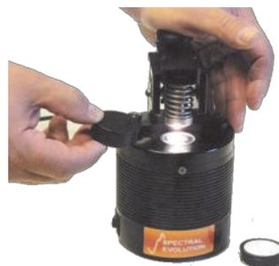
*An optional benchtop contact probe with sample soil compactor is useful for lab-based measurements.*
