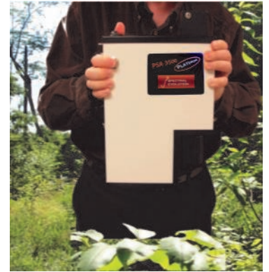
The PSR-3500 field portable spectroradiometer for remote sensing includes access to 19 vegetation indices
