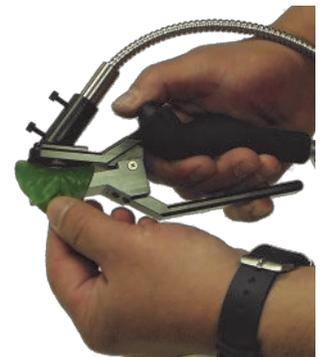
*Our unique leaf clip has an external trigger and a remote light source that makes it easy to use in the field and keeps heat away from your sample for better scans.*
