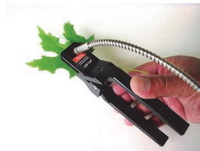
*The leaf clip includes a tungsten halogen light source and internal reference standard for ease-of-use and accurate measurement without affecting the sample.*
