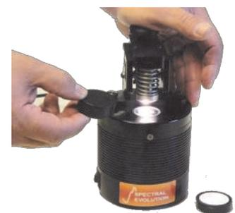
*An optional benchtop contact probe with sample soil compactor is useful for lab-based soil measurements.*
