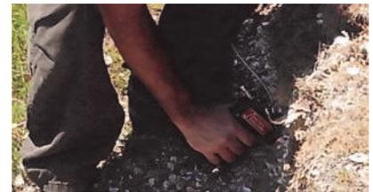
*Soil analysis using NIR spectroscopy can measure potassium, phosphorus, water, carbon, nitrogen, clay, pH, and organic matter.*
