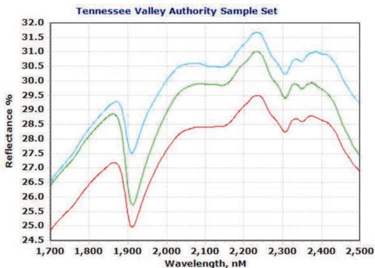
*Scans of coal samples from the Tennessee Valley Authority of high grade anthracite samples taken with an SR-6500 showing hydrocarbon features at 2300-2500 wavelengths.*
