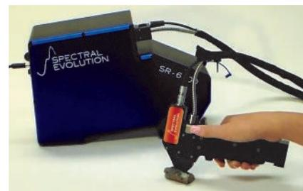
*SR-6500 delivers the highest available resolution for a portable spectrometer with a three TE-cooled photodiode array design.*
