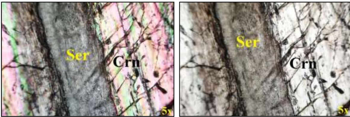
Fig.2. Bigger size Corundum under PPL and XPL
