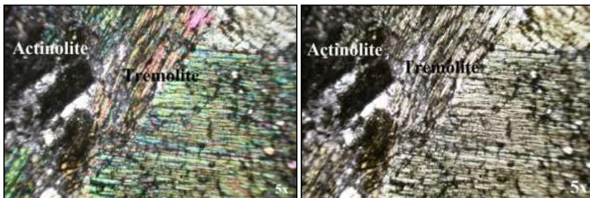
Fig.5. Actinolite Tremolite Schist under PPL and XPL
