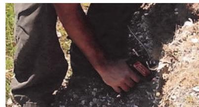
*Soil analysis using NIR spectroscopy can measure potassium, phosphorus, water, carbon, nitrogen, clay, pH, and organic matter.*
