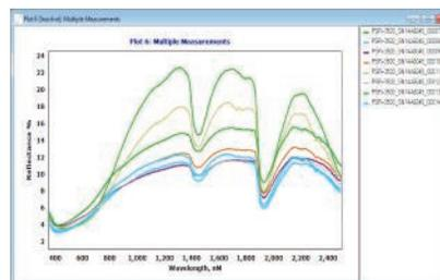
*DARWin SP Data Acquisition software allows you to display multiple scans for comparison and saves as ASCII files for use with chemometrics software*
