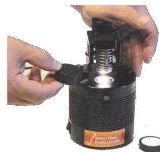
*An optional benchtop contact probe with sample soil compactor is useful for lab-based soil measurements.*
