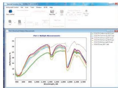
*DARWin SP Data Acquisition software is included with every SPECTRAL EVOLUTION spectroradiometer. The software allows you to display multiple scans of different soil samples for comparison.*
